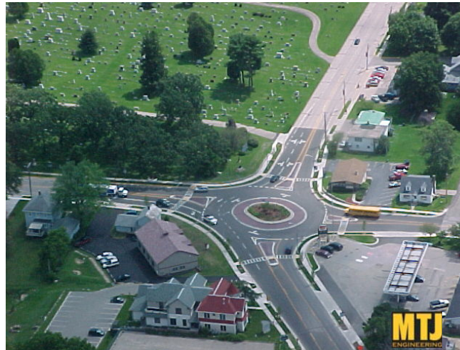
Mt. Horeb, WI: First Roundabout on WI State Highway Urban Compact Multi-Lane (3,000 VPH Design Year Flow)
