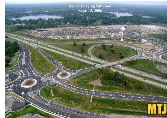
US 23 Lee Road, Michigan: Most Complex System of Roundabouts in US (7,800 VPH Design Year Flows)
